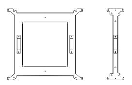
For quick installation of the videowall it's advised to use this spacer kit (not supplied). For each model of monitor there is a specific spacer kit available.
