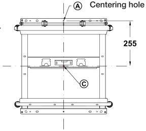
**2.2** Fix the bracket horizontally by using the holes (F) with a suitable anchor for your kind of wall.
