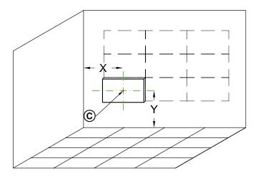
2.2 Mark 252 mm up from (C) to the centering hole (A).
