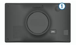
To put the device in power saving mode, press the power key while the device is on.
