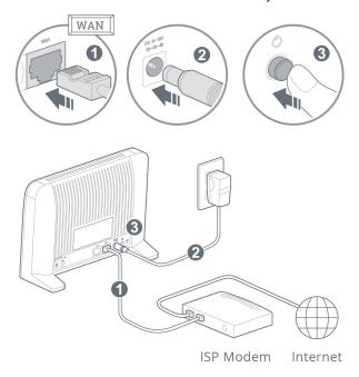
2 Connect one end of the power adapter to the power port on your MR2200ac, and the other end to the power outlet. Press the power button to power on your MR2200ac. Wait for around two minutes until the STATUS LED indicator starts blinking blue.
