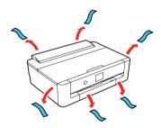
2 Open the printer cover and remove all protective materials from inside the product.
