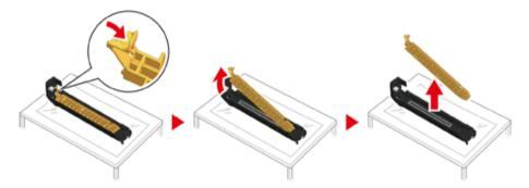
11 Insert the toner cartridge (7) removed in step 7 by aligning its left side indentation (8) with the protrusion (9) on the image drum so that the toner cartridge and image drum color label align. Then insert the right side gently into place.
