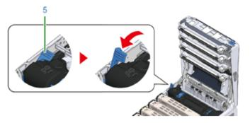
5 Hold the fuser unit handle (6) and take out the fuser unit from the machine.
