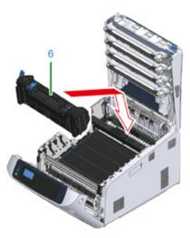
Push the left lock lever (5) of the fuser unit backward.
