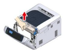
Take out the duplex unit (3) by pulling it obliquely upward while holding the center recess on the back of the machine.
