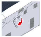
Pull out the connector, and plug it into the Wireless LAN module.
