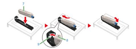
Turn the toner cartridge lock lever (blue) (10) of the toner cartridge backward until its top align on the ▶ mark while pressing the toner cartridge to attach the toner cartridge to the image drum.
