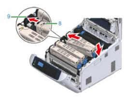
Holding the toner cartridge, turn the toner cartridge lock lever (5) (blue) all the way to the end in the direction of the arrow and lock the toner cartridge to the image drum.
