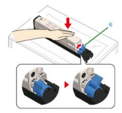
Check the label color of the new image drum and place the drum into the machine.
