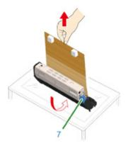
Put the image drum with the protective sheet removed into the printer unit and turn the toner cartridge lock lever (7) (blue) in the direction of the arrow until it clicks.
