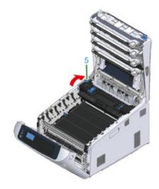
12 Return all four image drums into the machine carefully.
