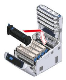
7 Push back the left locking lever (5) of the fuser unit to lock.
