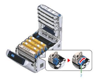
• Closing the cover without turning the toner cartridge lock lever (blue) may cause a malfunction. Make sure to turn the cartridge lock lever all the way to the other end side.
