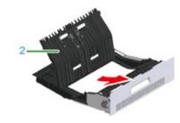
Replace the duplex unit (1) into the machine.
