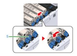
Lift the toner cartridge (6) from right side, and remove it from the machine.
