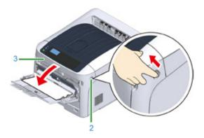
Remove the jammed paper gently by pulling the edge of paper.
