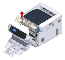
Remove the paper from the back gently if the edge of paper cannot be seen.
