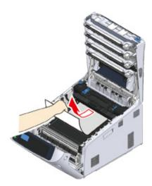
Pull out the jammed paper gently while lifting the release levers (5) on the fuser unit if an edge of jammed paper cannot be seen.
