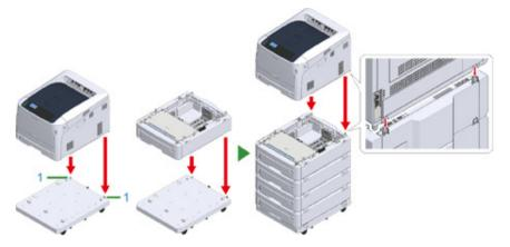
When attaching the additional tray unit, connect the printer unit and the additional tray unit.
