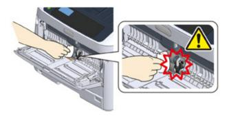
Open the separation roller cover (6) forward while pressing the center part of the MP tray.
