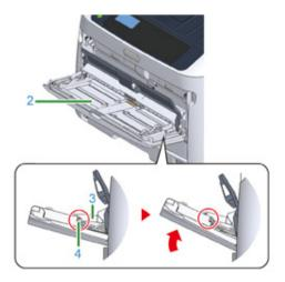
In the same manner, slightly lifting the MP tray (2), press the left arm (3) inward, then unlock the tab (4).
