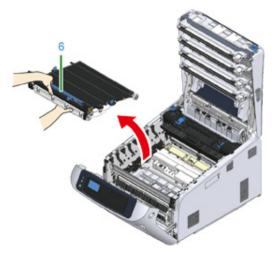
Hold the blue handle of a new belt unit, support the bottom of the belt unit, and insert the axis of the belt unit into the groove (7) in the printer.
