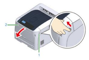
2 Remove the jammed paper gently in the direction of the arrow if an edge of jammed paper can be seen.
