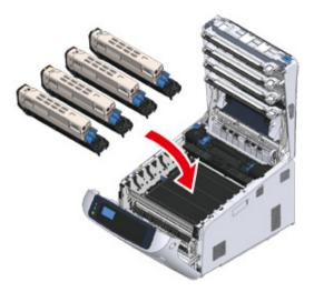
7 Close the output tray (4) by pushing the center of the cover firmly.
