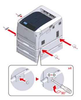
When attaching the caster base, lock the casters and set the tip-over protection tools.
