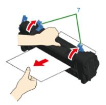
If jammed paper remains in the machine, hold the both sides of the paper to remove it gently.
