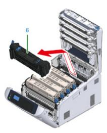
Hold the handle and place the new fuser unit into the machine.
