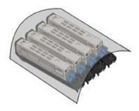
5 Pull out the jammed paper gently to the rear of the machine (the direction of the arrow) if an edge of jammed paper can be seen.
