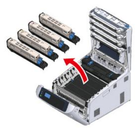
4 Cover the removed image drums with paper so that the image drums are not exposed to light.
