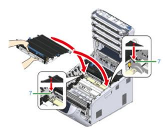
Q Lower the handle side of the belt unit and set the belt unit to the machine.
