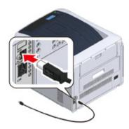
Insert one end of the USB cable into the USB interface connector on the machine.
