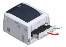
2 Check for jammed paper inside the machine. If jammed paper remains, remove it.
