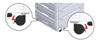
You can find two tip-over protection tools on the left and right sides of the caster base, and also two tools on its back side. Pull them straight out, then turn them  $90^{\circ}$  counterclockwise until they click.
