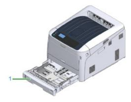
2 Set the paper size dial (2) to match the size of the paper to be loaded. Set the dial to [A4□] when loading A4 size paper in horizontal orientation.
