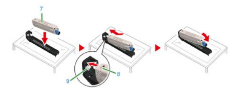
Turn the toner cartridge lock lever (blue) (6) of the toner cartridge backward until its top align on the ▶ mark while pressing the toner cartridge to attach the toner cartridge to the image drum.
