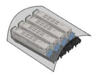
Turn the blue knobs (5) on each side of the belt unit in direction of the arrow to unlock.
