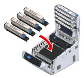
2 Close the output tray (4) by pushing the center of the output tray firmly.
