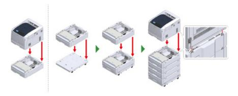
3 Screw the printer unit and the additional tray unit.
