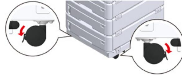
You can find two tip-over protection tools on the left and right sides of the caster base, and also two tools on its back side. Pull them straight out, then turn them 90° counter-clockwise until they click.
