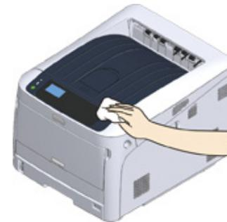
**3** Dry the surface of the machine with a dry soft cloth.
