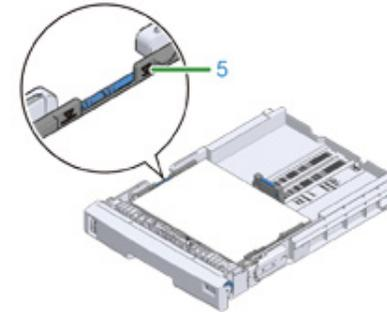
**6** Secure the loaded paper with the paper guide.
