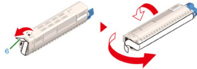
**11** Insert a new toner cartridge (7) by aligning its left side indentation (8) with the protrusion (9) on the image drum so that the toner cartridge and image drum color label align. Then insert the right side gently into place.
