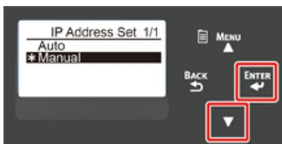
If obtaining the IP address automatically, check that [Auto] is selected, and press the «ENTER» button. Proceed to the step 16.
