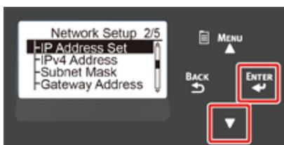
If setting the IP address manually, press the scroll button ▼ and select [Manual], and press the «ENTER» button. Proceed to the step 10.
