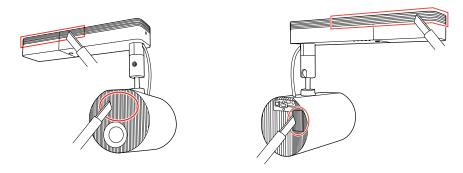
**Caution:** Do not use canned air. The gases may leave a flammable residue or push dust and debris into the projector's optics or other sensitive areas.
