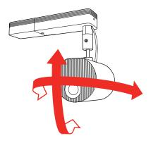
**Caution:** Make sure the cables do not tangle around the ball joint or you may damage the projector.
