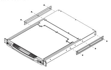
2. Attach the left and right *easy-installation* mounting rails to the inside of the rack. The flange that supports the switch will be to the inside.
