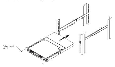
4. Slide the rear attachment sliding brackets along the slide bars until they contact the rear of the switch, then use the screws supplied with this package to attach the bars to the rear of the switch (tighten the screws all the way).
