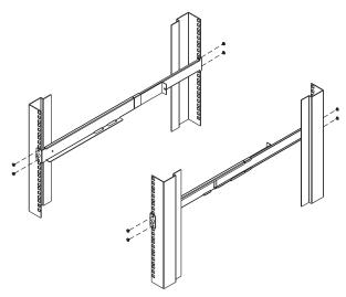
3. Slide the switch onto the support flanges. Use the screws supplied with this package to loosely attach the front of the switch to the front of the rack (only tighten the screws part way).
