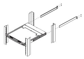
3. After the L brackets have been secured, tighten the front bracket screws.
