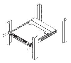
While the first person still holds the switch in place, the second person slides the L brackets into the switch's side mounting brackets, from the rear until the bracket flanges contact the rack, then screws the L brackets to the rack.
