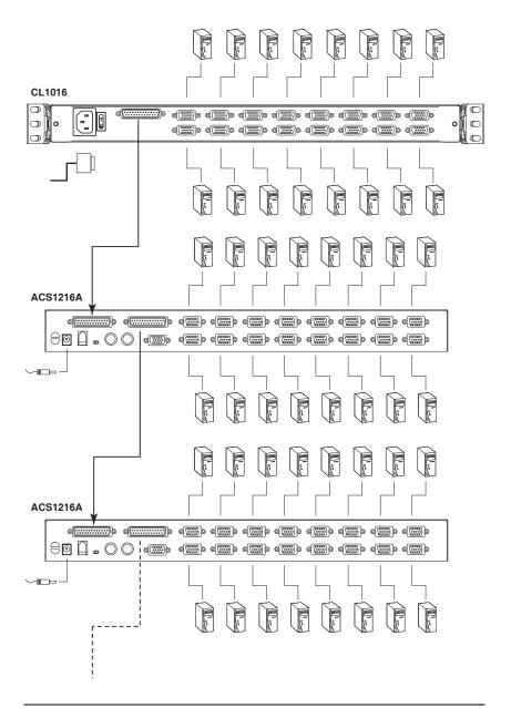
**Note:** The CL1016 is pictured above. The CL1008 rear panel is the same as that of the CL1016, except that it has 8 KVM ports instead of 16.
