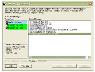
Check Firmware Version - when selected the utility compares the Main Board firmware level with the upgrade files MAIN. If the device versions are higher than the upgrade versions a dialog box informs you and gives you the option to continue or cancel.
