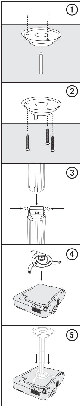
You have bought a ceiling mount for a projector. For mounting on concrete and wooden ceiling, please use the included screws and plugs. For mounting on other type of ceilings, please use intended screws and plugs (not included).
