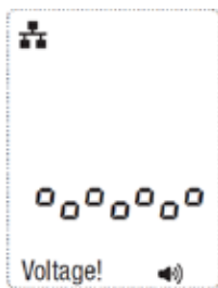
Data Cable, High Voltage detected! Disconnect immediately to prevent damage to the tester
