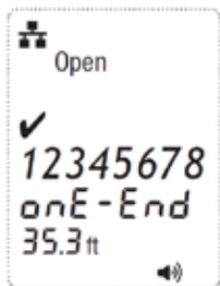
PASS, Data Cable, Single-ended test, shielding not tested, 35.3 ft
