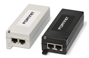
The single-port GPI-115 and GPI-130 Power over Ethernet (PoE) injectors offer a compact and cost-effective, fully IEEE 802.3af/802.3at-compliant solution to power FortiAP™ wireless access points and other compliant devices. They deliver single-port, mid-span, with 15.4/30 Watts of Gigabit Ethernet (GE) PoE, giving you maximum deployment flexibility.
