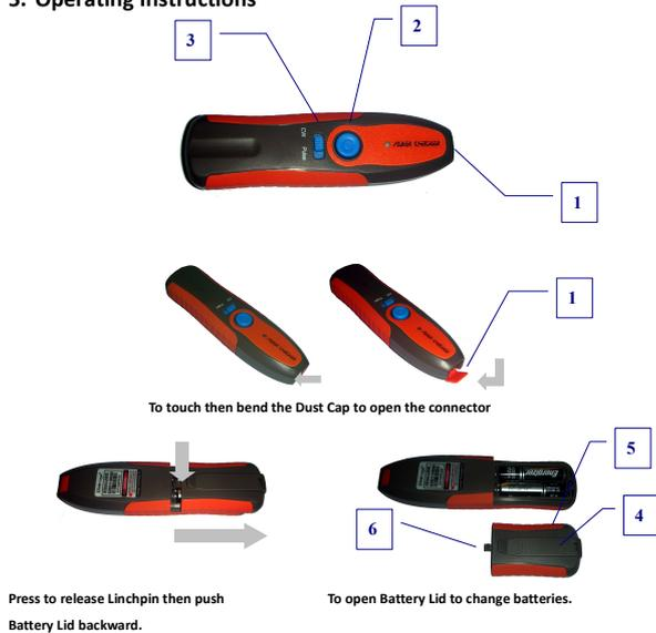
1. **Dust Cap** : prevents dirt contamination of the LD connector. To prevent the laser come out when turning on the power.
