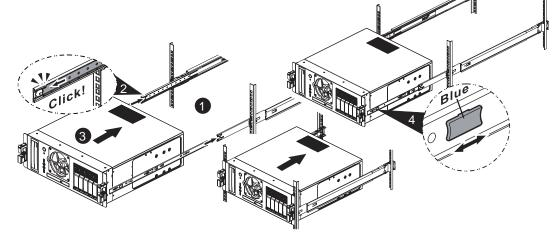
5) Remove the chassis from the rack.
