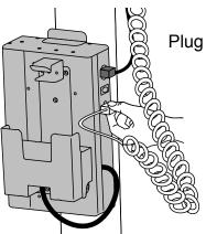
Plug coiled cord into wall outlet to charge battery.
