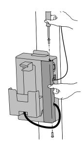
Route power strip from inside enclosure down to power module.
