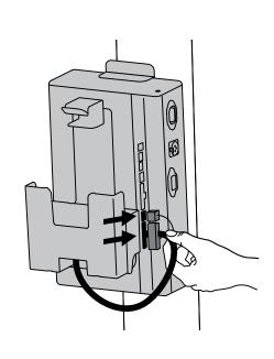
a Attach SOCI to worksurface, then route cable down and plug into power module.
