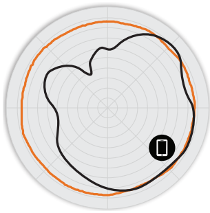
Figure 2. R610 2.4GHz Azimuth Antenna Patterns
