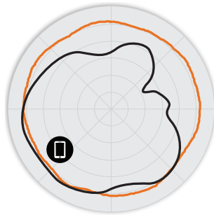
Figure 3. R610 5GHz Azimuth Antenna Patterns
