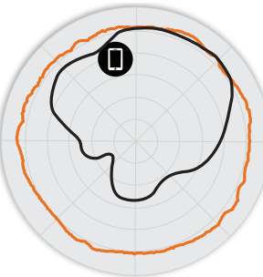
Figure 3. T301n 5GHz Azimuth Antenna Patterns
