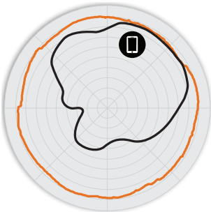
Figure 2. T301n 2.4GHz Azimuth Antenna Patterns
