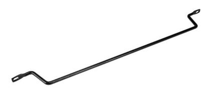
These lacing bars install horizontally on the front or back of your rack to provide a secure mounting point for you to run cables. You can attach your cables to the lacing bars using cable ties to reduce the tension on your cables and prevent damage to the ports on your rack-mount equipment. The lacing bars feature a 2 in. offset for hassle-free cable access.
