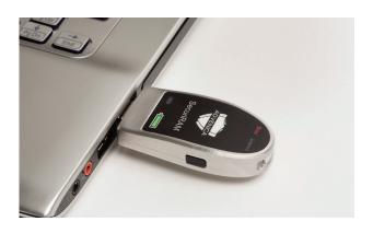
performing a secure erase on SecuriRAM once the information has been transferred to the untrusted system, any existing malware will be completely erased and the device can immediately be re-used.
