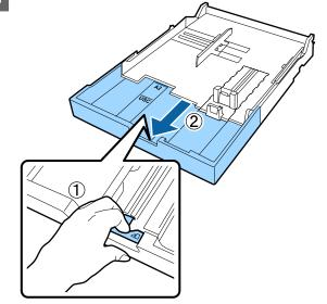
When extending the paper cassette, pull the lever in the paper cassette while extending. It locks in place when the lever is released.
