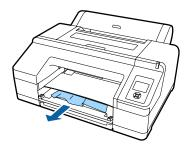
3 If paper is jammed in the rear, remove the rear unit by pulling it towards you with the knob moved to the inside as shown in the figure, and then remove the jammed paper.
