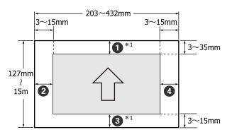
The margins for roll paper differ as shown below, depending on the **Roll Paper Margin** setting in the Menu.
