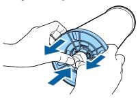
If the flange does not come off easily, lightly tap the end of the spindle on the black flange side.
