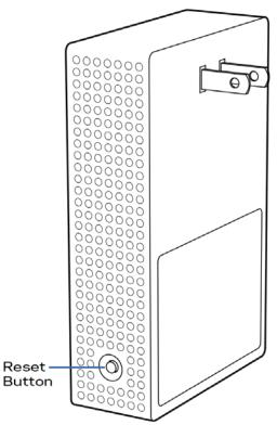
**Reset button**—Press and hold until the light on front of the node turns red, fades and flashes bright red again to reset the node to its factory defaults.
