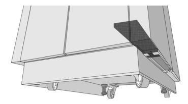
Slot the dustfilter foam into the front of the frame.
