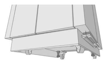
Align the opening in the metal frame with the air intake apertures on the undersides of the sidepods.
