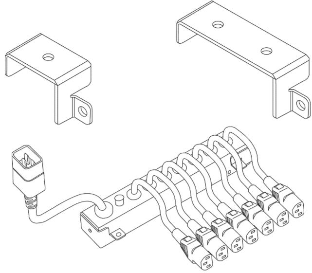
Each end of the stick shall provide an internal 5 mm nut (for attaching external mounting brackets). The brackets shall both fit on the stick with either a configuration of one stick per set of two brackets with the single bracket or with a configuration of two sticks with the double brackets. The brackets are shown above for reference. Actual dimensions can be found in the reference specifications.
