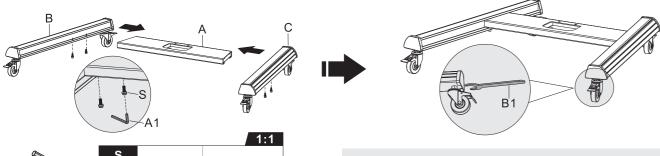
**Note:** Each caster can be adjusted independently for fine tuning. Slightly turn the nut to lower or raise the base.
