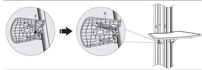
Put the hook&loop through the holes to fix the wrench.
