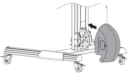
Align the clips on the plastic coves with the slots on the column until they snap shut onto the wire spool.
