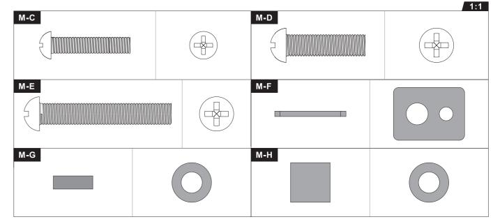
Note: Choose the appropriate screws, washers and spacers (if necessary) according to the type of screen.
