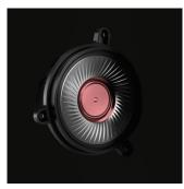
Layered Motion Control (LMC) drivers feature a multi-layered polymer diaphragm that encases a layer of damping gel. These layers form a flexible boundary and – together with the gel – absorbs and dampens any exaggerated frequencies, resulting in a smooth and flatter frequency response. The result is a more balanced, natural and refined range of high frequency sounds.
