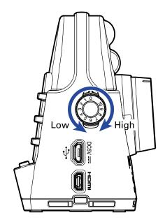
Adjust so that the level meters are around –12 dB with the loudest sounds.
