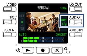
Press **DELAY** again repeatedly to lengthen the audio delay time.
