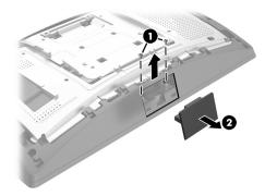
Insert the USB connector on the LCD module into the top USB port ①, and then secure the module with the two screws that were previously removed ②.
