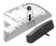
4. Align the tabs on the display head rear cover with the slots on the display head. Place the cover on the display head, and then slide the cover down so that it snaps into place.
