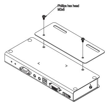
2. Screw the bracket into any convenient location on the rack.
