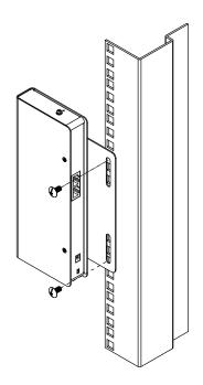
**Note:** These screws are not provided. We recommend that you use M5 x 12 Phillips Type I cross, recessed type screws.
