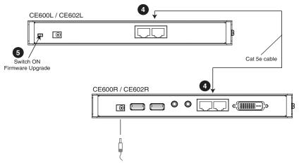
6. Plug in the Local Unit's power adapter to power it on.
