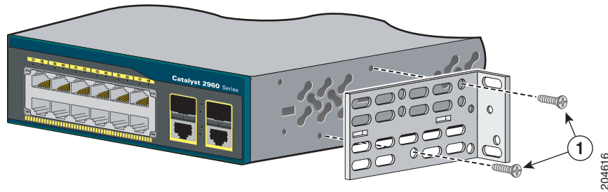
Figure 2-6 Attaching Brackets for 19-Inch Telco Racks to a Catalyst 2960 Switch
