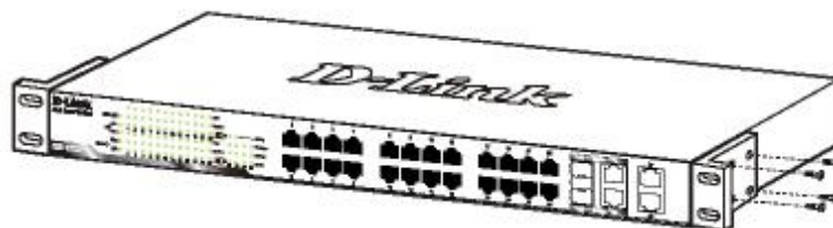
Figure 2 – Attach the mounting brackets to the Switch
