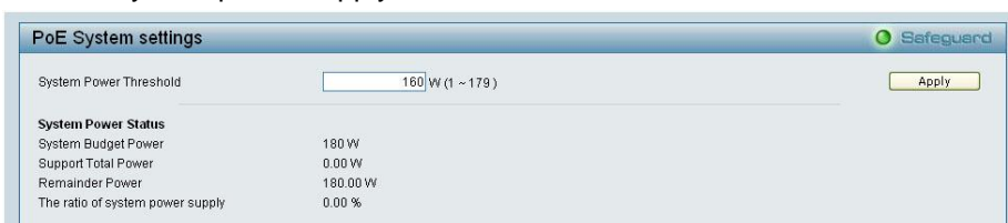
Figure 63 – PoE > PoE System Setting
