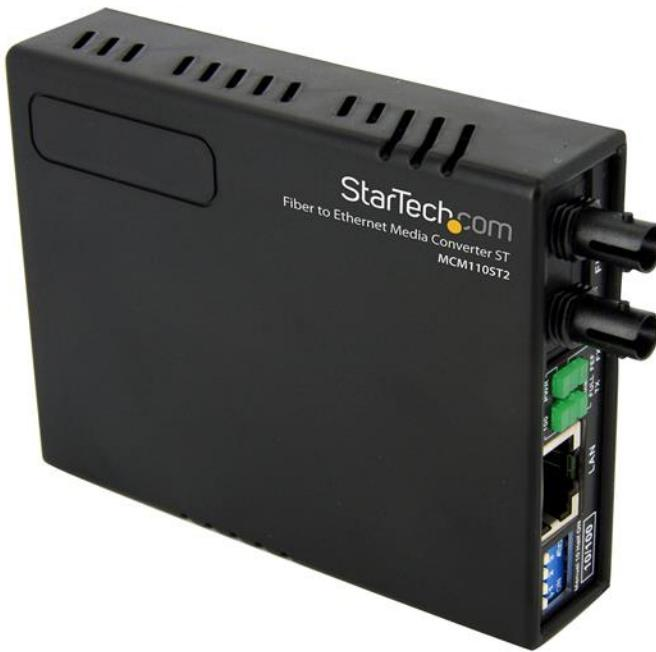
The MCM110ST2EU 10/100 Multi Mode ST Fiber Ethernet Media Converter (2 km) creates a cost-effective Ethernet to fiber link, transparently converting to/from 10Base-T or 100Base-Tx Ethernet signals and 100Base-Fx optical signals to extend an Ethernet network connection over a multimode fiber backbone.
