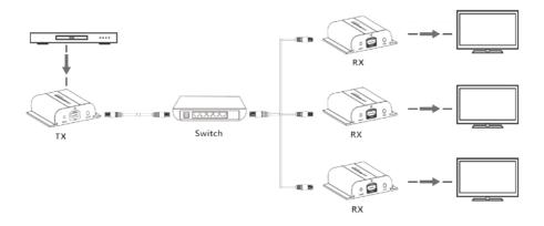
NOTE: Multicasting uses more bandwidth. Vision recommends using a standalone Gigabit switch. It can be an unmanaged switch since IGMP snooping DOES NOT need to be activated.
