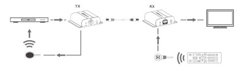
1.2 CONNECT VIA NETWORK. By routing via the network there is no cable length limitation as the signal is repeated at every node.
