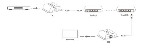
NOTES: All items must be on same subnet. Microwave transmitters typically do not provide enough bandwidth for this product. 18Mbps per receiver required.
