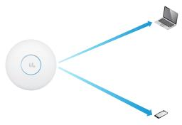
MU-MIMO with 3x3 and 1x1 clients: The UniFi AC SHD AP communicates with one 3x3 client and one 1x1 client at a time.
