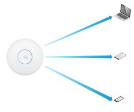
MU-MIMO with 2x2 and 1x1 clients: The UniFi AC SHD AP communicates with one 2x2 client and two 1x1 clients at a time.
