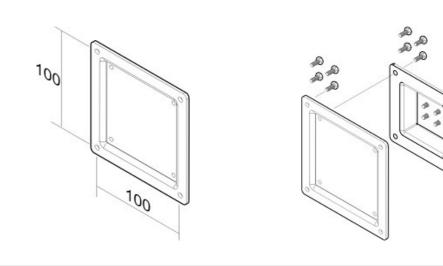
This adapter allows you to convert the hole pattern of your LCD TV mount. It converts hole patterns from VESA 75x75 to 100x100. Ideal to mount larger LCD/TFT monitors to wall-, desk- and ceiling mounts.
