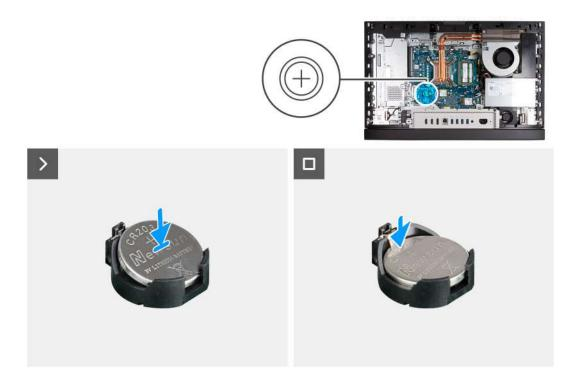
With the positive-side (+) facing up, insert the coin-cell battery into the battery socket on the system board and snap the battery into place.
