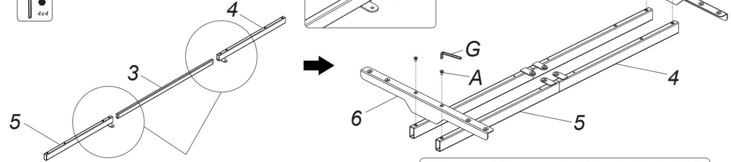
Using screws (A) to connect the connection rod (3) with the left supporting beam (4) and the right supporting beam (5), and tighten them with the allen key (G).
