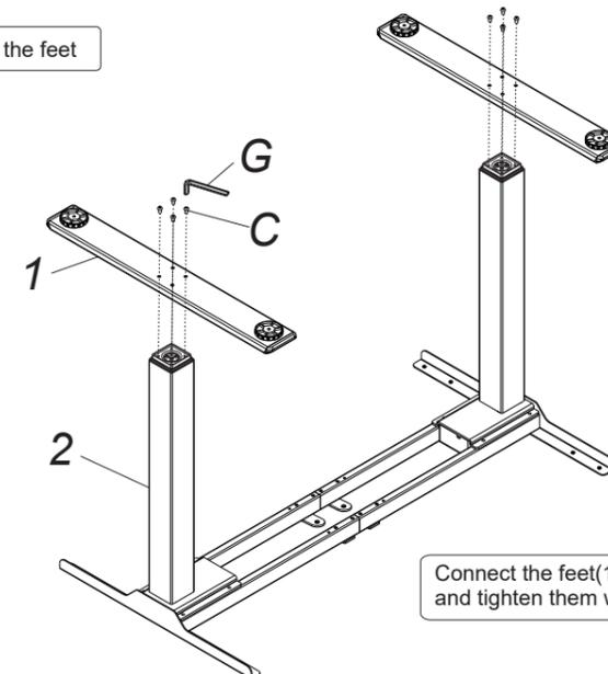
Connect the feet(1) and the lifting column (2) with screws (C), and tighten them with the allen key (G).
