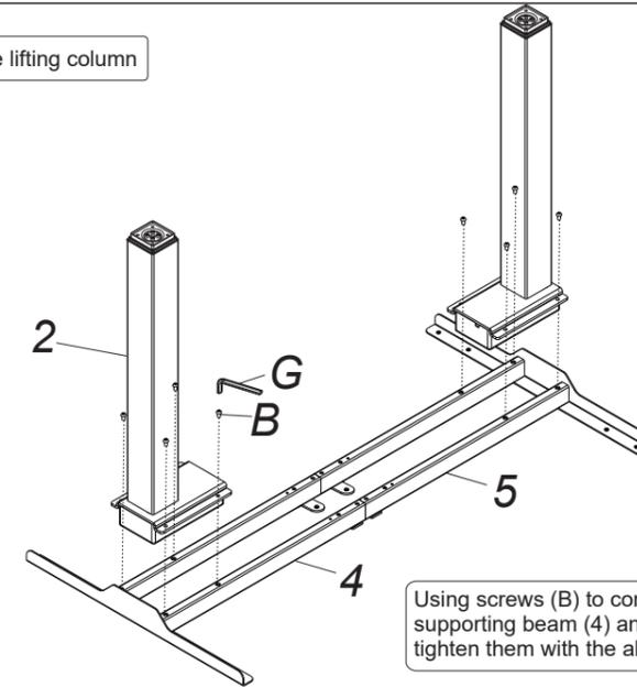
Using screws (B) to connect the lifting column (2) with the left supporting beam (4) and the right supporting beam (5), and tighten them with the allen key (G).
