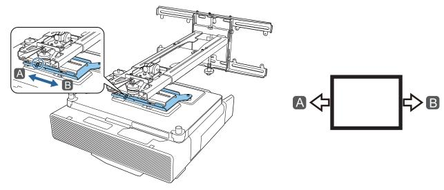
Loosen the M4 bolts (x2), and then adjust the forward/backward slide
