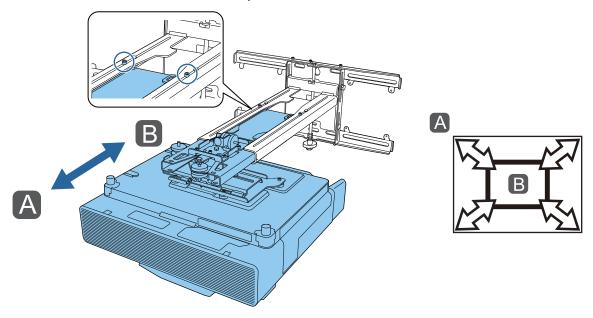
Loosen the M6 bolt, and then adjust the vertical slide
