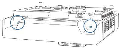
Loosen the M4 bolt on the adjustment unit, and then align the marks for each part
