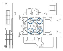
Attach the adjustment unit to the setting plate with the M4 x 12 mm bolts (x4) supplied
