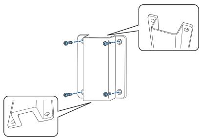
Place the AC adapter in the holder and connect it to the power supply
