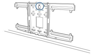
Use commercially available M10 or 3/8 inch x 60 mm anchor bolts to secure the wall plate to the holes you drilled in step 4
