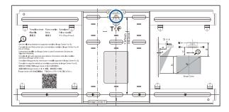
Determine the positions for the mounting holes for the wall plate
