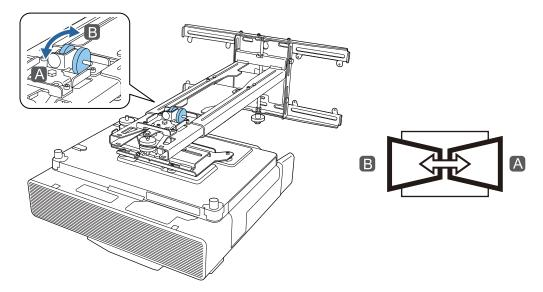
Turn the adjustment dial 3 in the installation guide to adjust the vertical tilt
