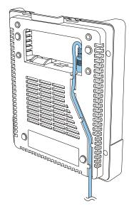
Check the installation position and secure with commercially available M4 screws (20 mm x4)
