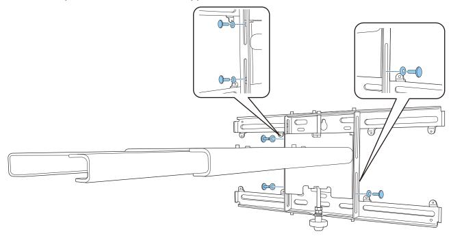
Adjust the vertical slide with the open-ended spanner to align the marks on the wall plate and the setting plate.
