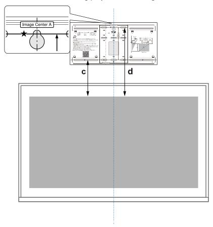
Drive a commercially available M10 screw into the position of the temporary screw hole for the wall plate
