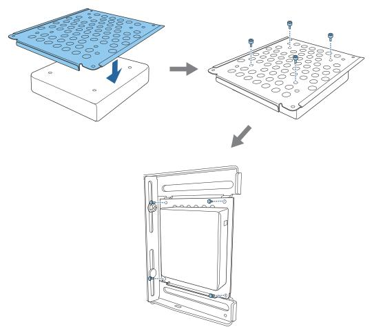
• Secure the mini PC plate to the wall plate using the M3 x 6 mm screws (x4) supplied, and then install the PC.
