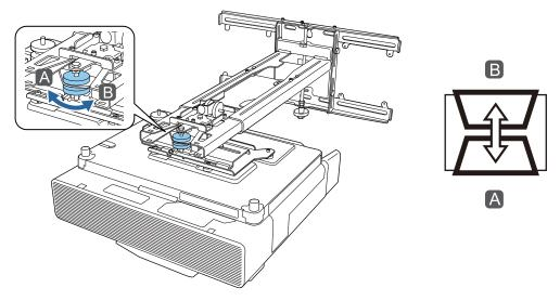
Loosen the M4 bolt, and then adjust the horizontal slide
