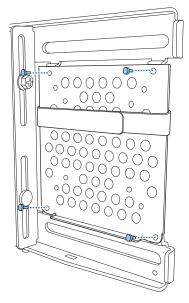
Place the PC on the lower edge of the mini PC plate, and secure it with the belt
