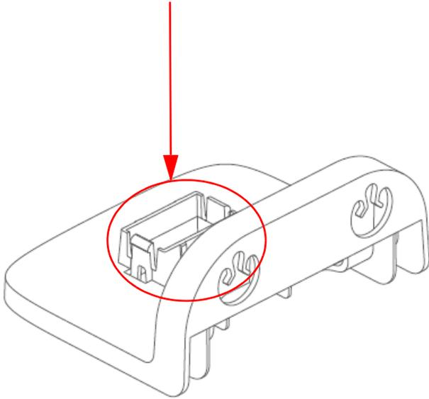
**Figure 12** Secure the WSM20 to the Mounting Base
