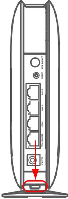
**Figure 14** The hook on the side panel B
