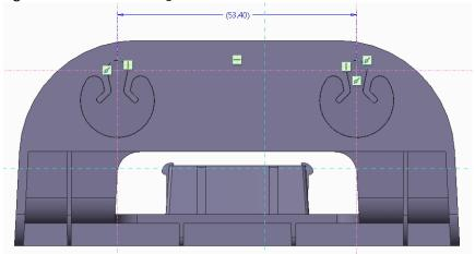
2 Insert the anchors and then screw the mounting base into the wall using the screws of the required specs as shown below.
