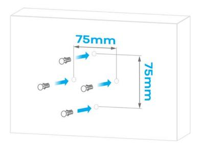
2 Screw the mounting base into the wall or ceiling.
