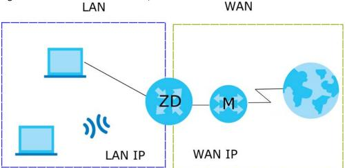
• Bridge Mode: In bridge mode, Multy M1 has one IP address and Multy M1 interfaces are bridged together in the same network. To see the bridge mode features, go to Table 8 on page 119. In the example scenario below, Multy M1 connects the local network to the Internet through a router (R).
