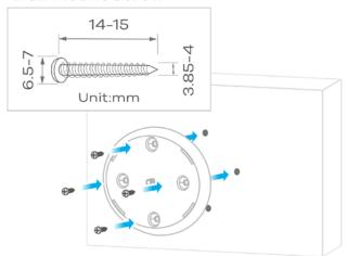
3 Line up the Multy's base hole with the mounting base screw. Gently turn the Multy clockwise until it is secured to the mounting base.
