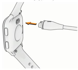
2 Plug the large end of the USB cable into a USB charging port. The watch displays the current battery charge level.
