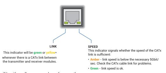
\* The CATx LINK LED will be either yellow or green, depending upon the connector manufacturer used. There is no difference in functionality.
