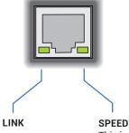
\* The CATx LINK LED will be either yellow or green, depending upon the connector manufacturer used. There is no difference in functionality.
