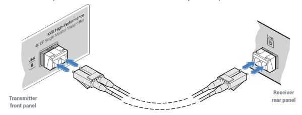
Note: In order to maintain a high level of confidence in the fiber optic link, it is recommended that Black Box supplied SFPs are used.
