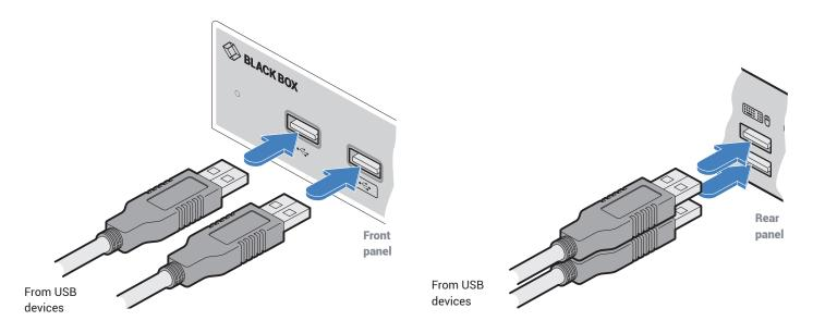
Note: [200-series models only] The front panel socket labeled is a fully transparent USB port capable of supporting a wider range of devices, such as headsets, web cams and flash drives.
