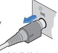
Gently pull back the plug outer body to release the lock
