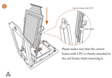
Install the carrier frame with CPU. Don't separate them.
