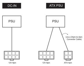
The following diagram illustrates how to connect the bundled ATX 24pin-to-4pin converter cable.
