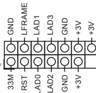
This connector supports Trusted Platform Module (TPM) system, which can securely store keys, digital certificates, passwords, and data. A TPM system also helps enhance network security, protects digital identities, and ensures platform integrity.
