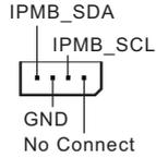
This 4-pin connector is used to provide a cabled base-board or front panel connection for value added features and 3rd-party add-in cards, such as Emergency Management cards, that provide management features using the IPMB.
