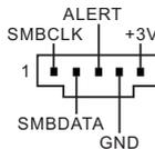
PSU SMBus monitors the status of the power supply, fan and system temperature.
