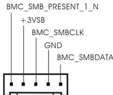
The header is used for the SM BUS devices.
