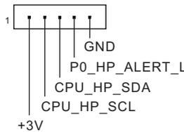
This header is used for the hot plug feature of NVMEs on the backplane.
