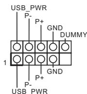
There is one USB 2.0 header on this motherboard. This USB 2.0 header can support two ports.
