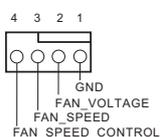
Please connect the fan cables to the fan connectors and match the black wire to the ground pin. All fans supports Fan Control.
