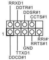
This COM header supports a serial port module.
