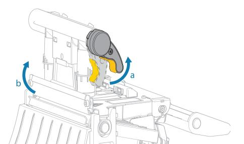
Rotate the printhead latch (a)
