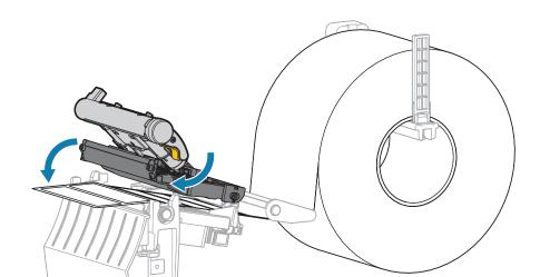
Rotate the printhead lever down to close the printhead.
