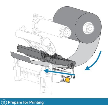
Wrap the ribbon around the core several times, and then rotate the spindle to tighten and align
