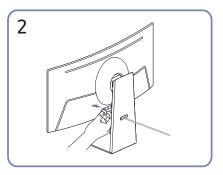
Connect the cables to the corresponding ports.
