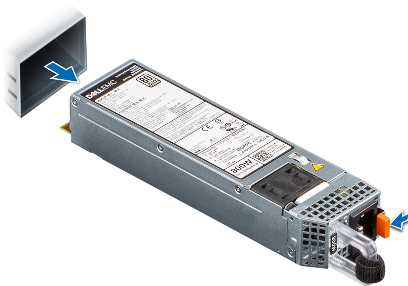
Figure 98. Removing a power supply unit
