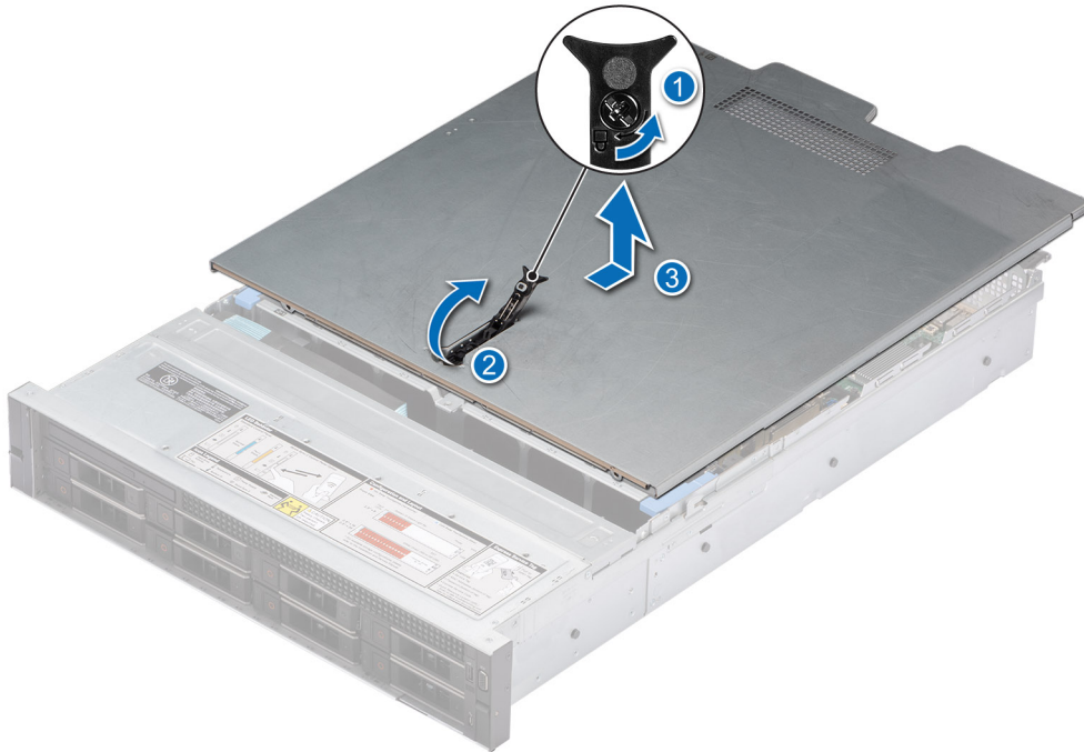
Figure 20. Removing the system cover
