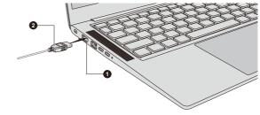
Figure 4-6 Connecting the HDMI™ out port
