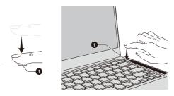
Figure 4-2 Using the Fingerprint Sensor
