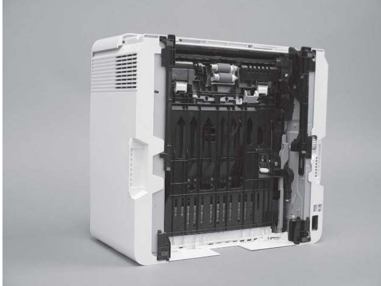
Figure 6-14 Place the printer bottom-side face forward
