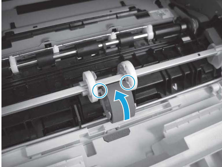
Figure 6-11 Install the roller
