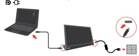
2) Connect Type-C power adapter to the left or right side of M14t and connect M14t to the mobile phone with a USB-C cable.
