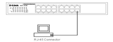
Switch connected to an end node
